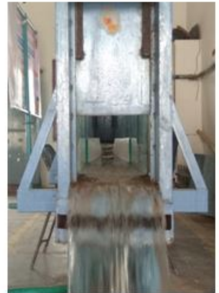
Front View of Trapezoidal Venturi Flume
