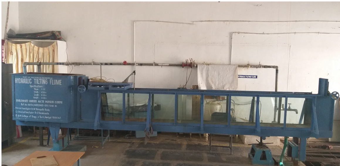
Figure 3.3: Hydraulic Tilting Flume
