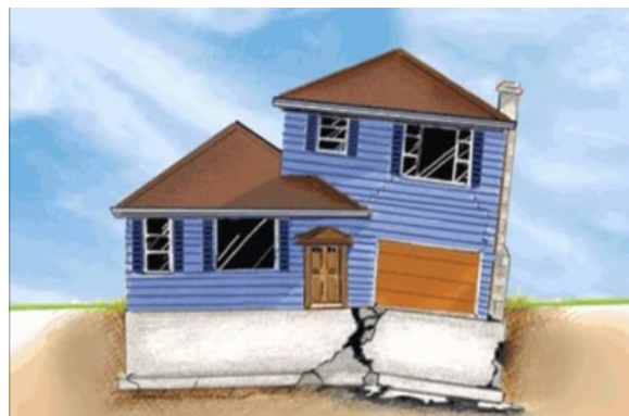
Figure 1.10: Differential Settlement of Foundation
