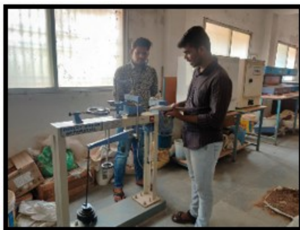
Figure 3.1: Direct Shear Test
