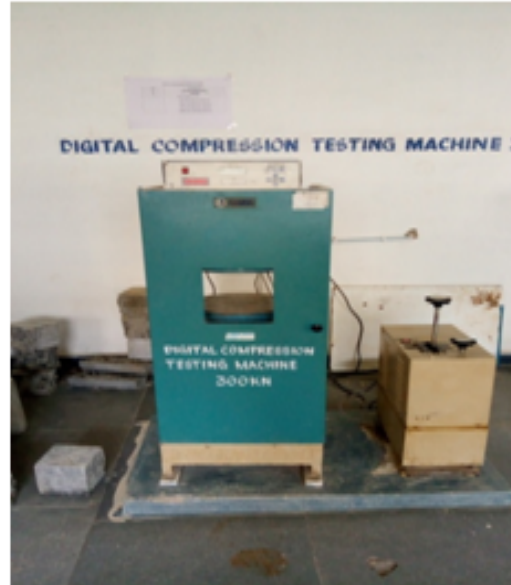
1 Digital Compression Testing Machine[3000KN]
